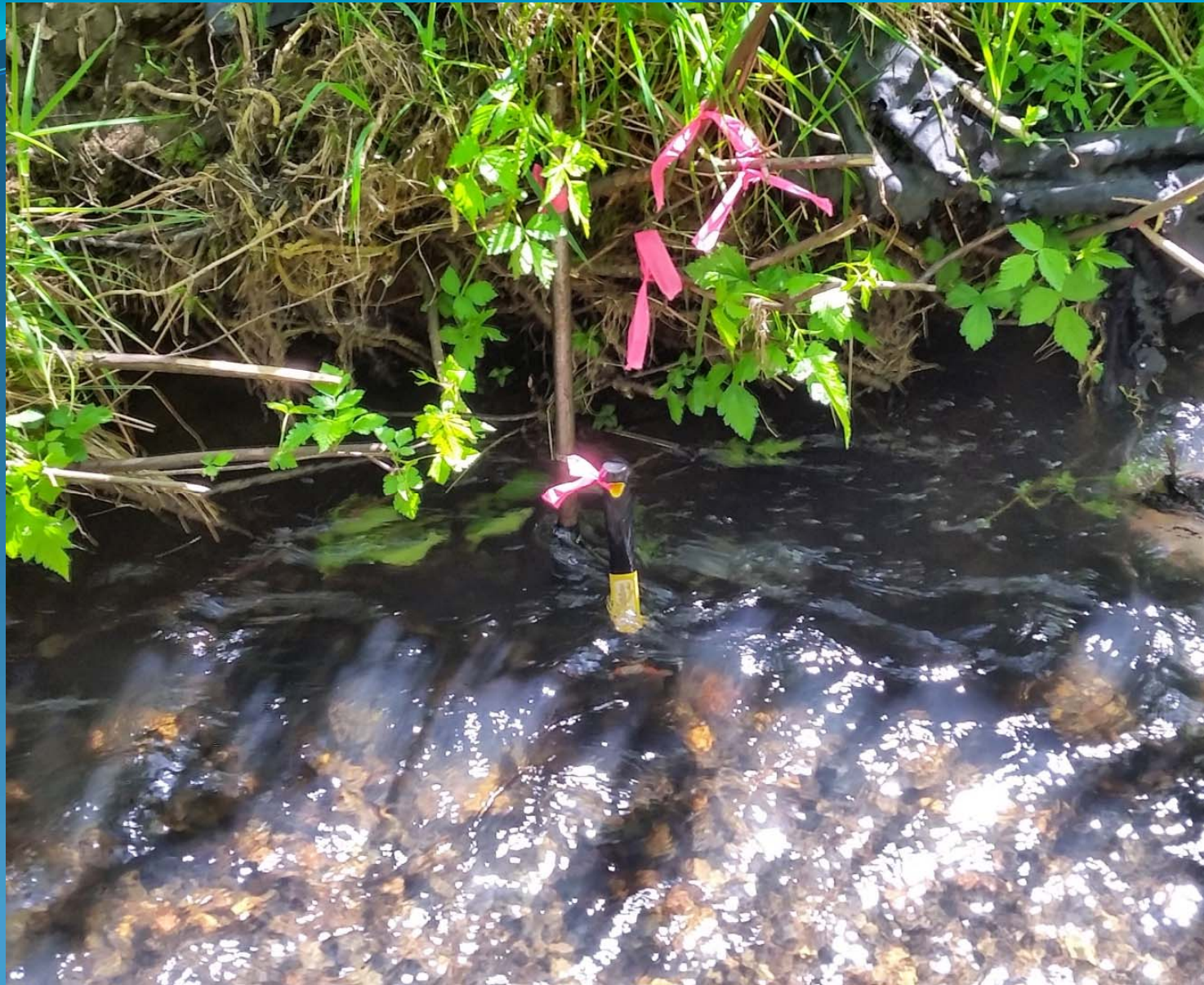
Temperature sensor/logger deployed in shadow near bottom of creek
