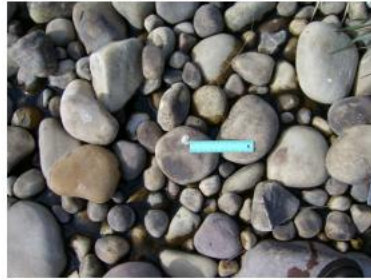
Photo of patch at NC site (blue 152mm ruler for scale): 50% cobble, 50% large gravel
