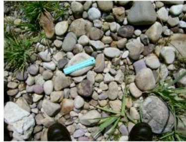
Photo of patch at NC site near PC#1 (blue 152mm ruler for scale): 30% cobble, 35% large gravel, 35% medium gravel
